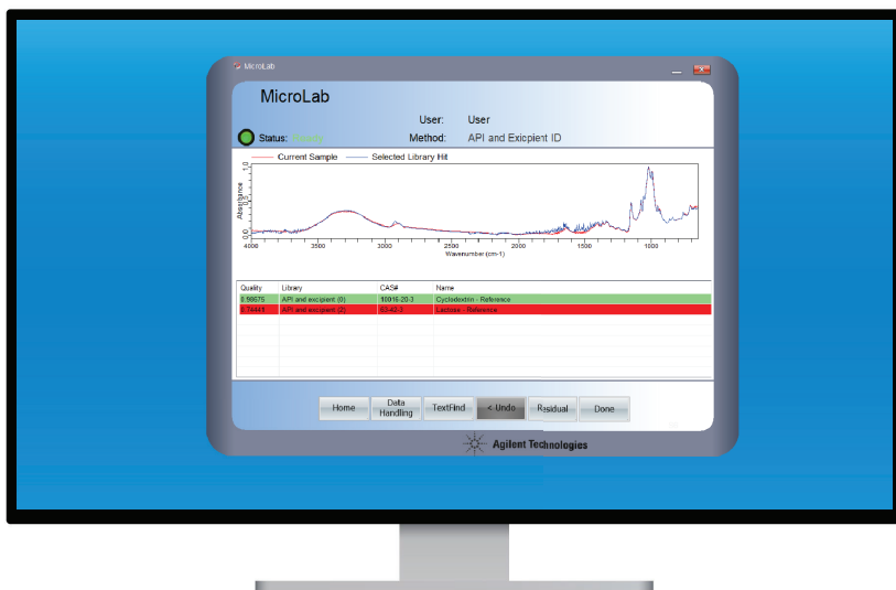
Figure 9. The Agilent MicroLab software applies color-coding to the library search results. Color-coding simplifies the interpretation of the results and reduces oversights that may lead to errors. The screenshot shows the results for \alpha -cyclodextrin in green, indicating a good match with the library spectrum.
