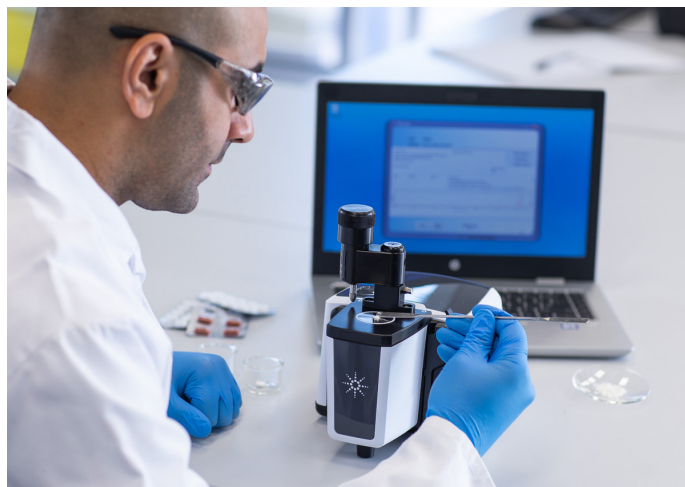
Figure 1. The Agilent Cary 630 FTIR with diamond ATR sampling module is used to establish the identity of different powders.
