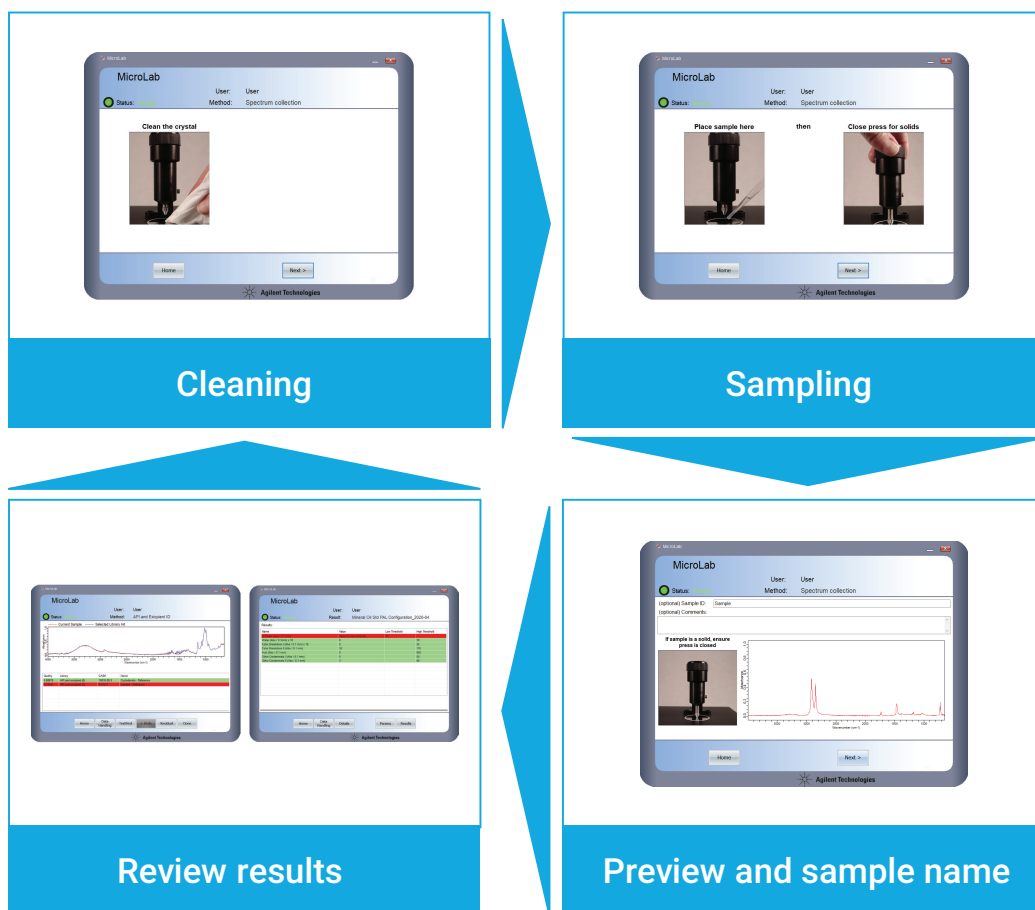
Figure 5. Agilent MicroLab software picture guidance interface simplifies performing an analysis using the Agilent Cary 630 FTIR, reducing training needs. The software replicates what the operator sees when using the instrument. After data acquisition, the results are directly displayed in an easy-to-understand format as shown in Figures 6 and 10. After the user has checked the results, the software starts the next analysis, ensuring a continuous analytical workflow.
