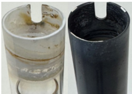
Example 2: During the analysis of 1.5% Li, Na, Cs in 5% HNO 3 solution, the quartz (left) shows significant devitrification after just 24 hours of analysis, whilst the ceramic outer tube-set (right) demonstrates its robustness with no obvious degradation after more than 900 hours of analysis.
