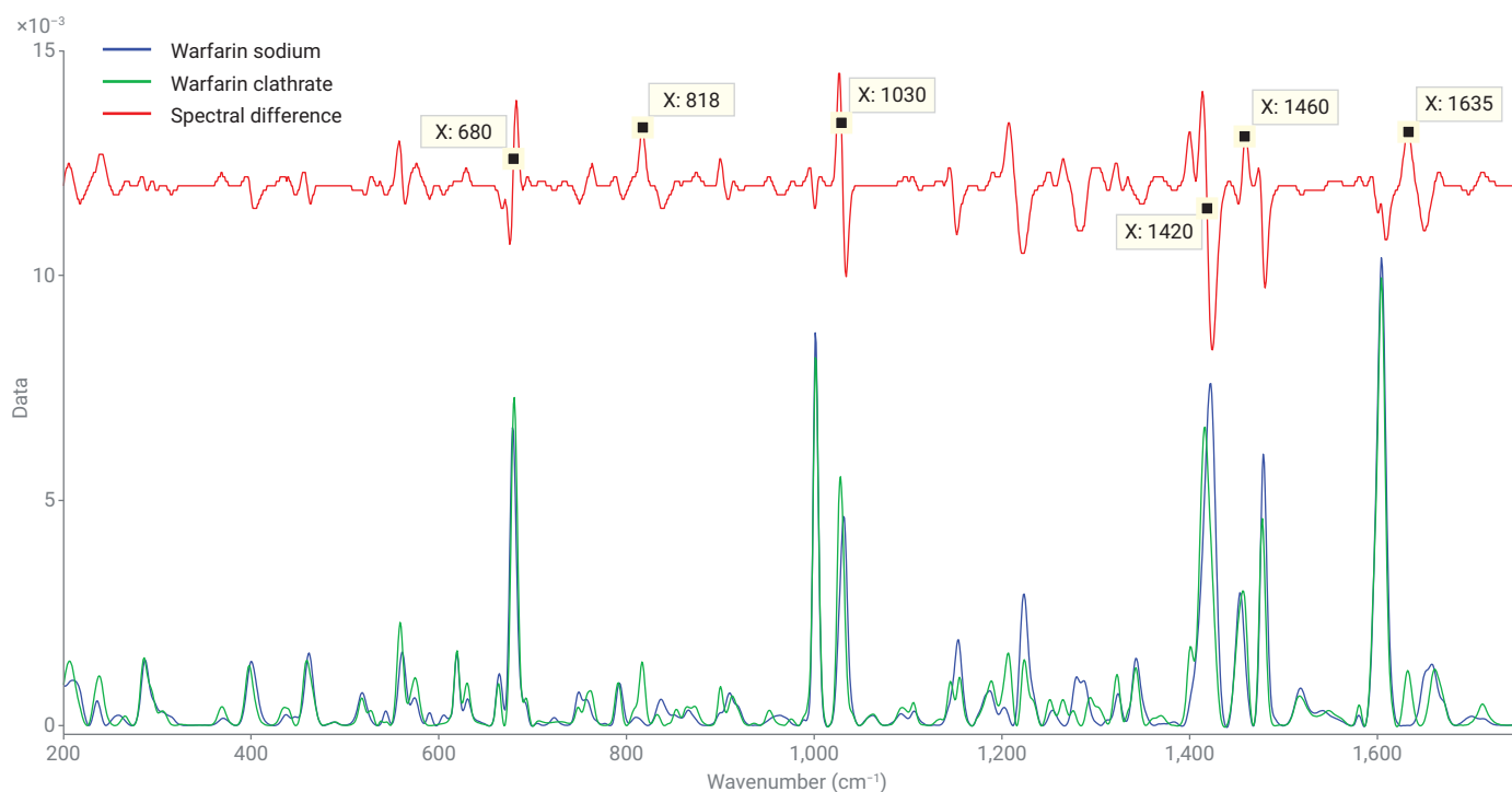
Figure 1. Warfarin sodium and Warfarin sodium clathrate transmission Raman spectra, with calculated spectral differences.
