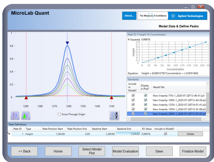
Figure 5. Linearity evaluation of the DialPath using MicroLab Quant software. Calibration curves and correlation coefficient calculations are performed automatically in the software. Users can report the obtained results for documentation purposes.
