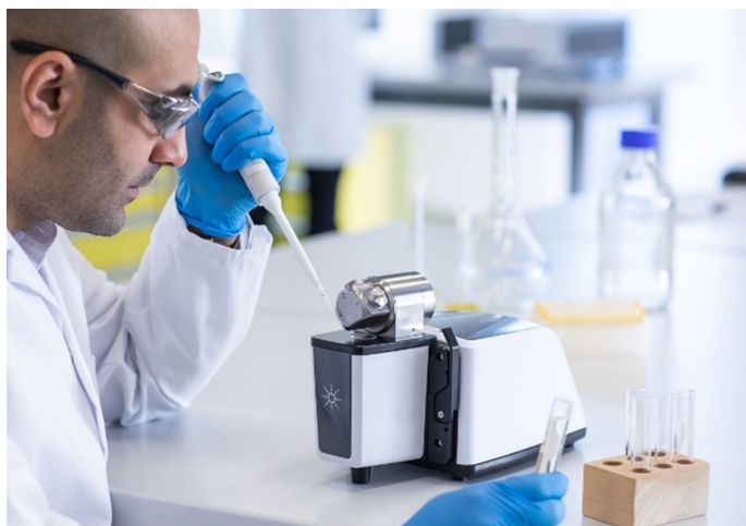
Figure 2. The liquid sample is placed onto the sample window of the DialPath module fitted to the Agilent Cary 630 FTIR spectrometer.
