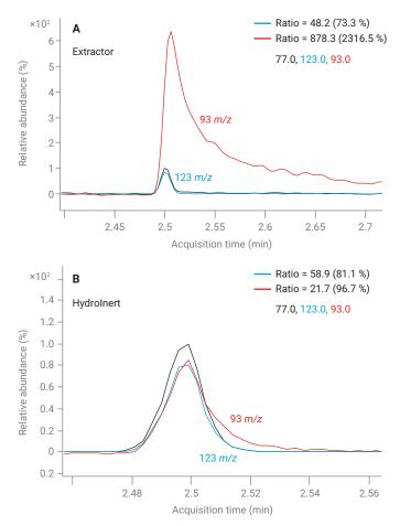
**Figure 2.** EICs of nitrobenzene with  $H_2$  carrier gas in (A) extractor source with 3 mm extraction lens showing hydrogenation to aniline with the abundant 93 *m/z* ion and (B) Agilent HydroInert source, showing an improved 123 versus 93 *m/z* ratio.
