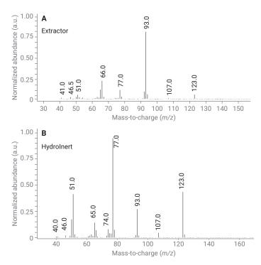
**Figure 1.** Mass spectra for peak eluting at nitrobenzene retention time with  $H_2$  carrier gas in (A) extractor source with 3 mm extraction lens showing hydrogenation to aniline with the abundant 93 m/z ion and (B) Agilent Hydrolnert source, showing an improved mass spectrum that correlates to nitrobenzene.
