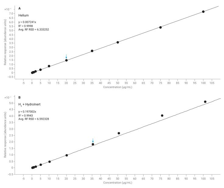
Figure 5. Nitrobenzene linear range (0.1 to 100 µg/mL) collected on a GC/MS system in (A) He and in (B) H<sub>2</sub> carrier gas with the Agilent HydroInert source.
