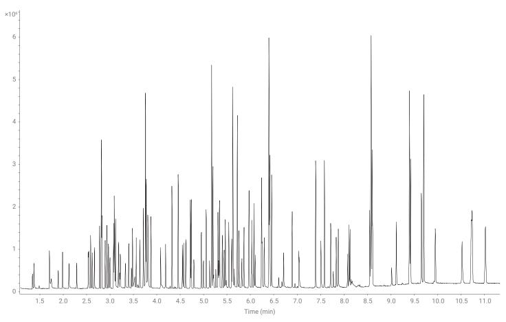
Figure 3. TIC of the 20 µg/mL calibration standard containing 119 target analytes and surrogates and six internal standards using H<sub>2</sub> carrier gas and the Agilent HydroInert source.
