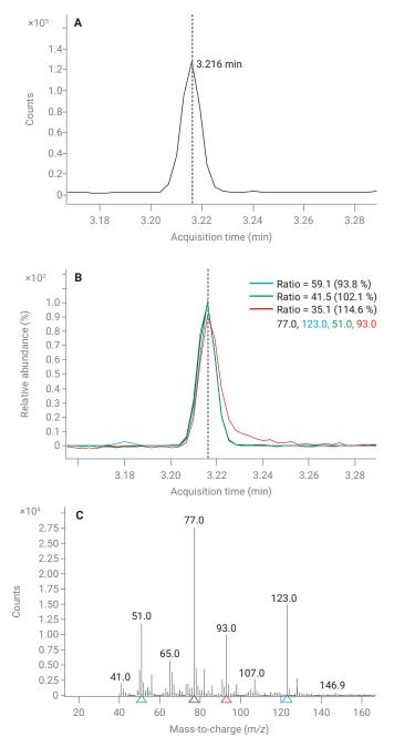
**Figure 6.** Nitrobenzene compound information for the 10  $\mu$ g/mL standard; (A) extracted ion chromatogram (EIC 77 *m/z*) of the base peak; (B) overlay of base peak (77 *m/z*) and top three qualifier EICs (123, 51, 93 *m/z*); (C) raw mass spectrum for nitrobenzene peak at 3.216 minutes.
