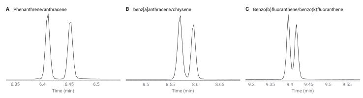
**Figure 4.** Midlevel standard (5  $\mu$ g/mL) EICs for critical isomer pairs: (A) phenanthrene and anthracene (EIC 178 *m/z*); (B) benz[a]anthracene and chrysene (EIC 228 *m/z*); (C) benzo(b)fluoranthene and benzo(k)fluoranthene (EIC 252 *m/z*).
