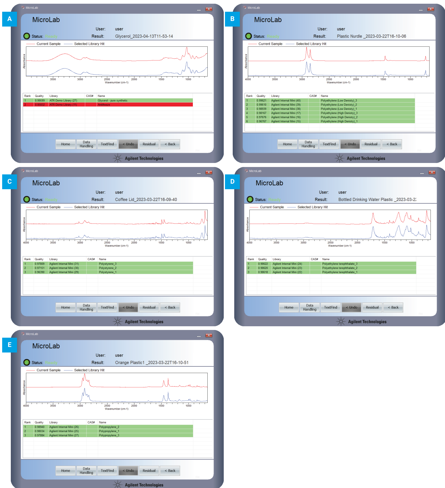
Figure 4. The Agilent Cary 630 FTIR spectrometer qualitative analysis of the five plastic samples (red traces) and library hits (blue traces). The table shows the hit quality, library used, and the hit name for each sample; (A) plasticizer; (B) nurdle; (C) coffee lid; (D) water bottle; (E) weathered plastic.
