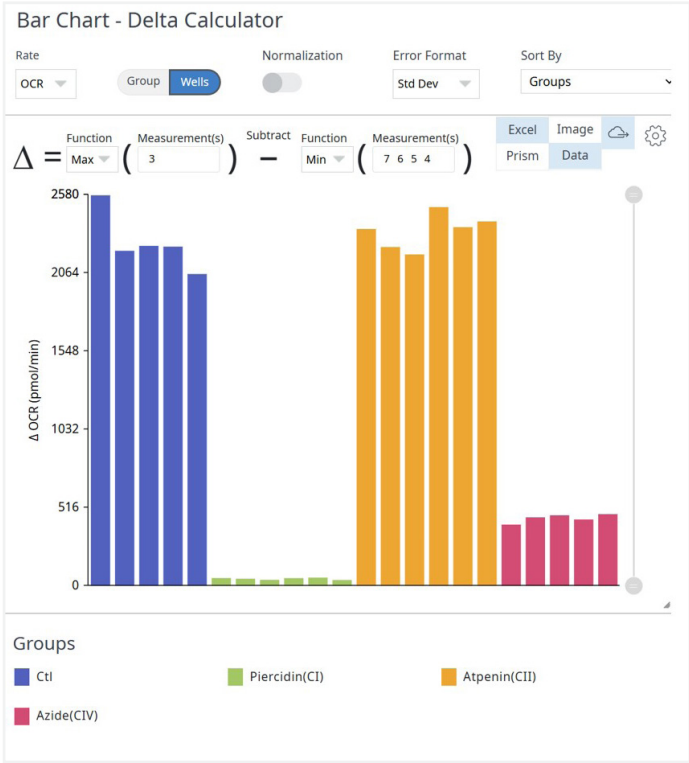
Figure 8. Bar Chart - Delta Calculator widget in Agilent Seahorse Analytics illustrating the well-wise calculation of OCR measurement 3 – OCR min (rotenone), the resulting value represents Complex I-linked respiration and can be exported to Microsoft Excel or Graph Prism.
