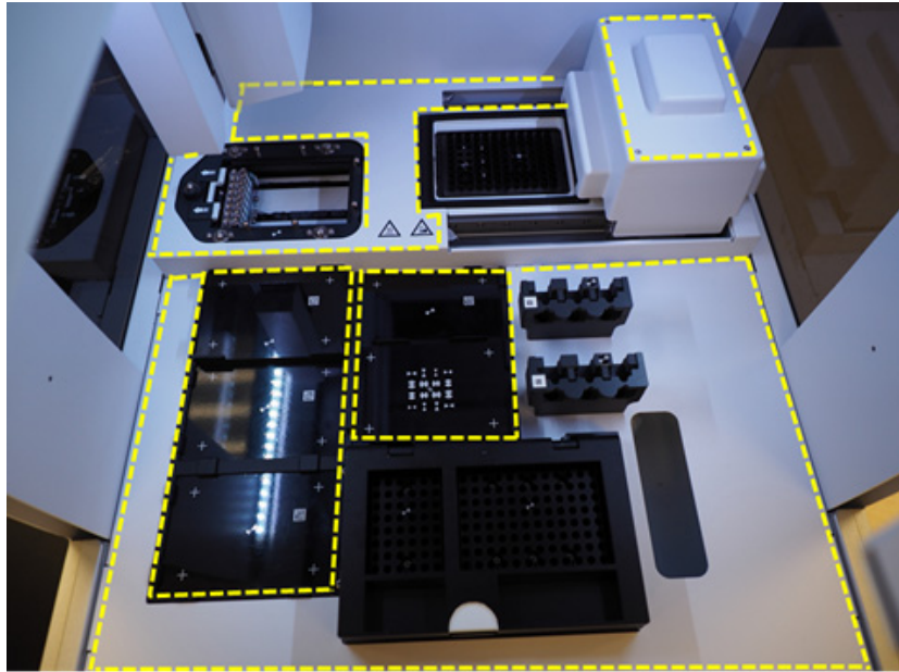
Figure 32 Deck surfaces to be wiped down
