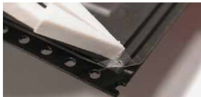
Figure 2. Removal of clear plastic covering
