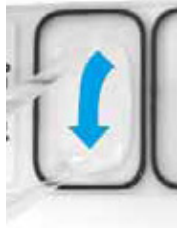
Figure 6. Drag and dispense method – Start dispensing when the pipette tip is near the top of the well. Finish dispensing when the pipette tip is near the bottom of the well.
