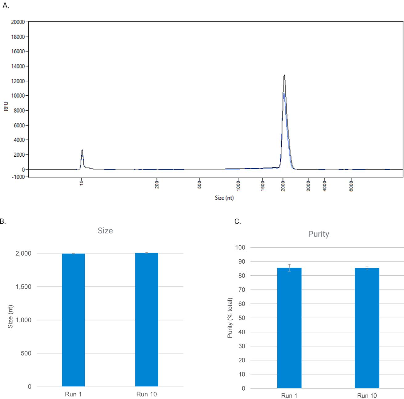
**Figure 5.** IVT mRNA samples prepared for analysis on an Agilent 5200 Fragment Analyzer system remained stable at room temperature for approximately 10 hours. A representative 2,055 nt IVT mRNA sample was analyzed over 10 subsequent runs, with no significant change in A) sample distribution, B) size, or C) purity, which was assessed using the percent total with a smear range from 1,800 to 2,400 nt.
