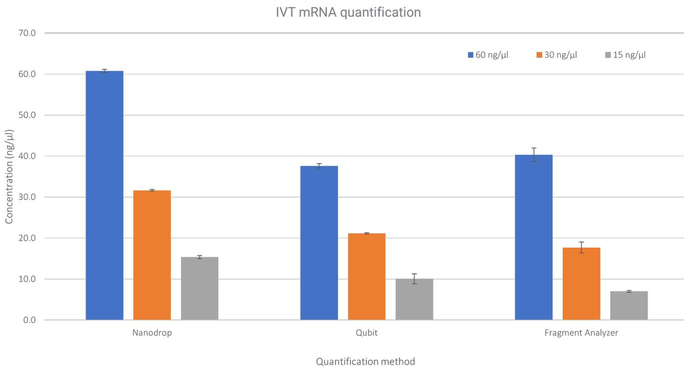
**Figure 7.** Reported concentration of a 996 nt IVT mRNA sample using the NanoDrop, Qubit, and Agilent 5200 Fragment Analyzer system.
