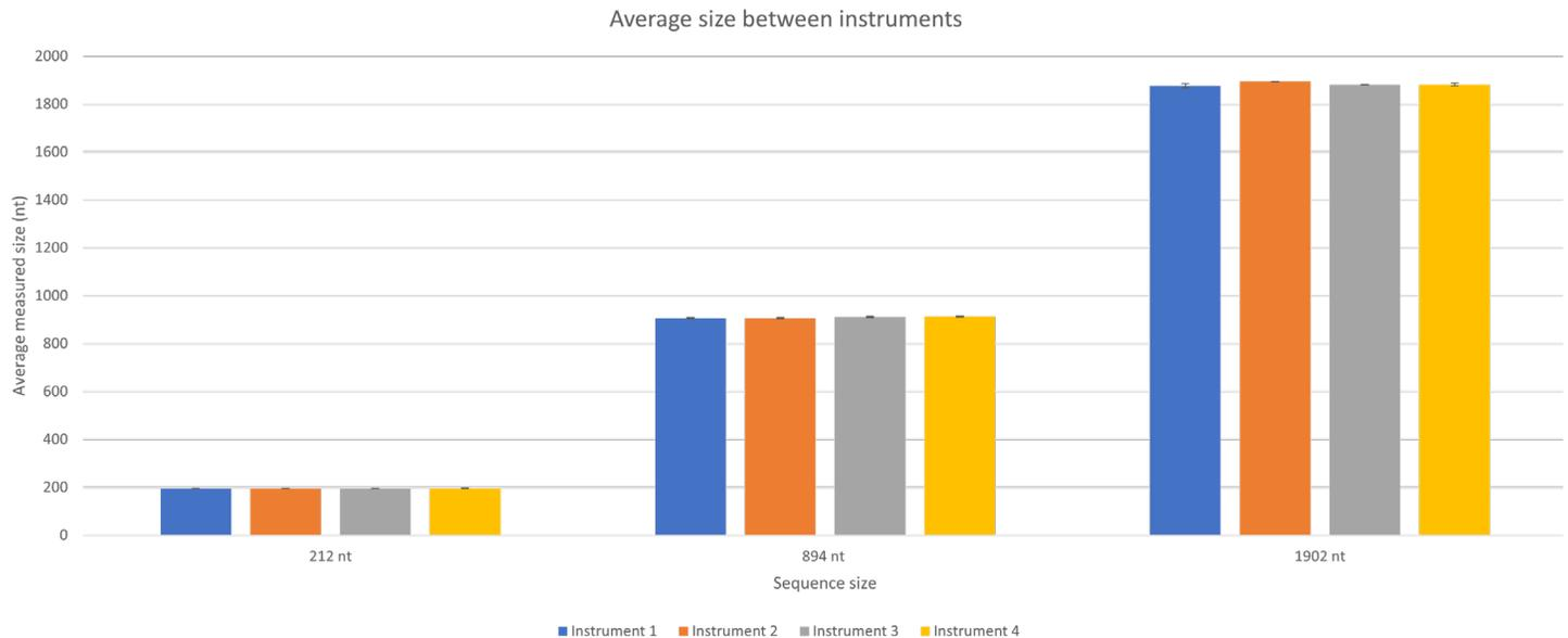
**Figure 6.** Three IVT mRNA samples of varying sizes were evaluated in triplicate across four Agilent 5200 Fragment Analyzer systems to demonstrate the ability of the instruments to provide reproducible analysis data. The average size of each fragment remained consistent across all instruments tested. Error bars show standard deviation.
