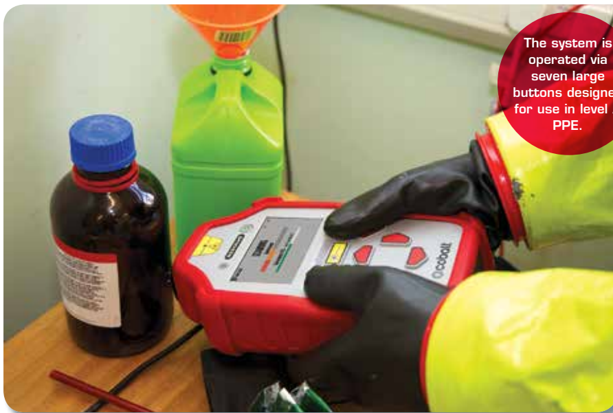
Resolve's through-barrier SORS technology works with coloured and opaque plastics, dark glass, paper and plastic sacks and envelopes as well as clear plastic bags and clear glass vials.
