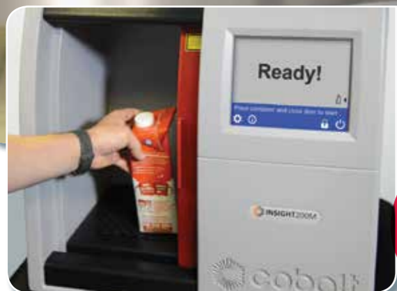
The Insight200M screens all containers, including metals (Tetra Paks are foil lined).
