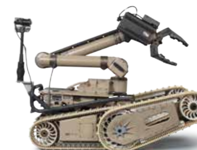
710 Kobra™ Counter-VBIED robot that lifts up to 330 lbs, reaches 11.5 feet height and sustains speeds of 8 mph
