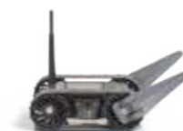
110 FirstLook® Five-pound throwable robot that provides eyes and ears for quick situational awareness
