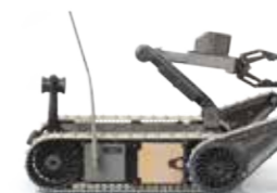
310 SUGV Lightweight, backpack portable, and easy-to-deploy robot for mobile operations
